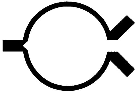
1.6 Directional couplers : their geometry is computed using a very accurate formulation (Kirschning & Jansen [4]) together with a Newton-Raphson optimisation routine. Effects like dispersion and end effect on coupled lines are taken into account. A coupler is typically computed and drawn in less than 30 seconds.
