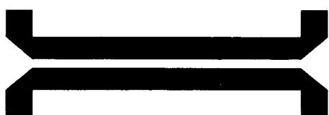
1.7 Quarter-wave transformer : automatically computed from the input and output impedances.
